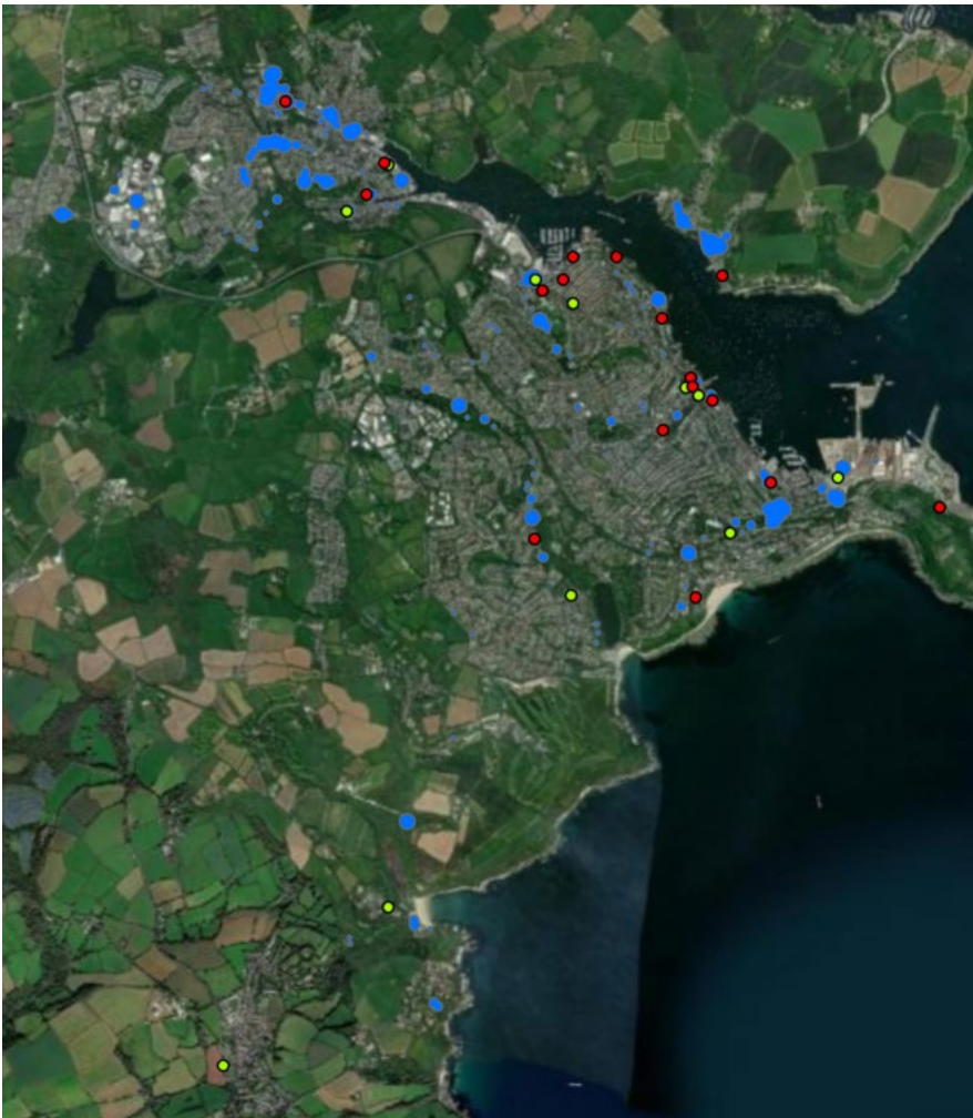
Figure 1: Baseline 2050 1:50 flood risk locations (blue) and storm overflow sites with more than 10 spills (red). Storm overflows that are already compliant with the Government spill targets are shown in green.
