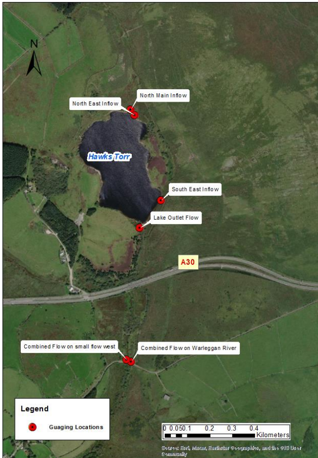
Figure 4.6 – Location of spot flow gauging undertaken by SWW in October 2022.
