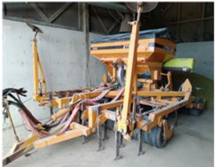
Simba Freeflow drill purchased by WRT for conservation tillage on the Otter
