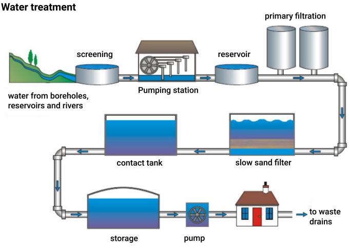
Water from boreholes, reservoirs and rivers is screened to protect fish, remove weeds and floating debris.
